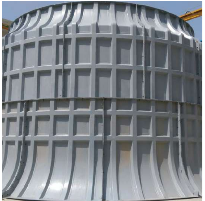
Two part fanstack manufactured and assembled at Arvind workshop
